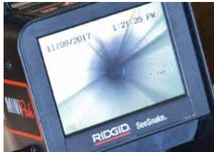
Daviesway DASC0's Shaun Kingston can check the entire milk line within minutes with an inline camera. Contract milker Brad Arnold has the box seat and he can clearly see the results on the screen (pictured above). Daviesway DASC0's service is free for all of its chemical customers.
