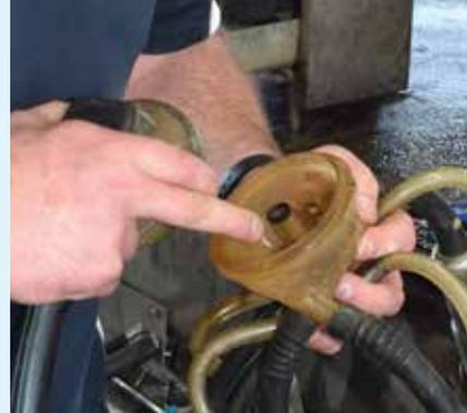
If the claws aren't clean, it points to a problem with water quality water temperature, or chemical not dosing correctly.
