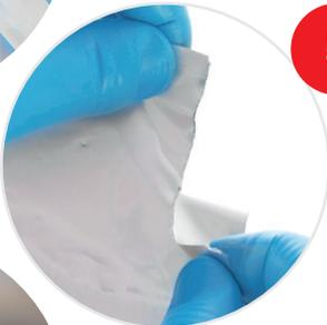
Tear the aluminium envelope open at the notch. Once the device has been taken out of the envelope its stability is of short duration, especially in a humid environment.
