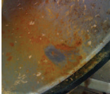
The combined build-up of iron in the water and milk solid residue in a milk receiveal can is hard to miss.
