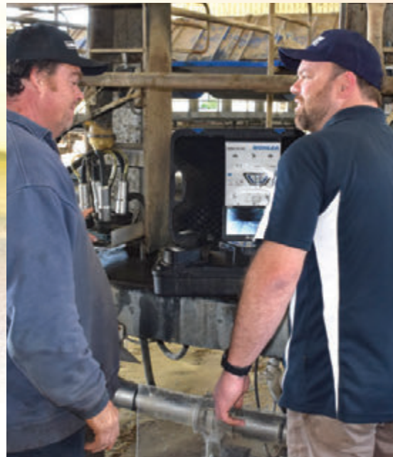
An inline camera allows DASC0's Peter Parniak to check the inside the entire milk lines within minutes.
