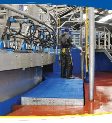
Adjustable floor level allows for different operators to select their ideal working level for claw attachment.
